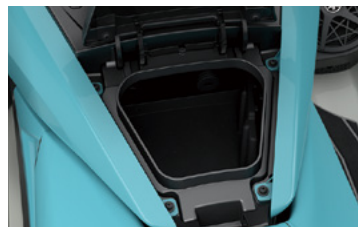
Glove Box Watertight with USB & 12V Outlet with Accent Lighting
