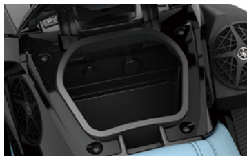
Watertight Glove Box with USB and 12V Outlet
